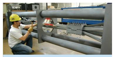
Wedges being driven into the cable sample
